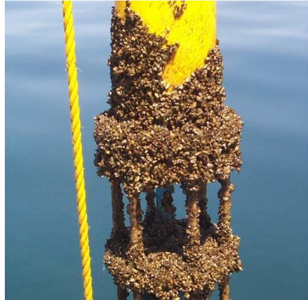
Current measurement instrument encrusted with zebra mussels
